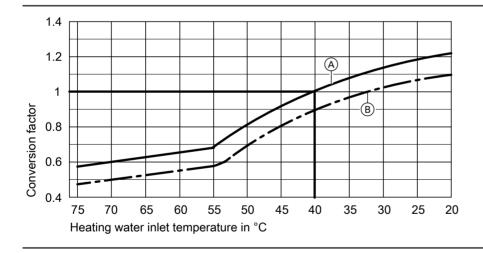
(A) Flue gas inlet temperature 200 °C
