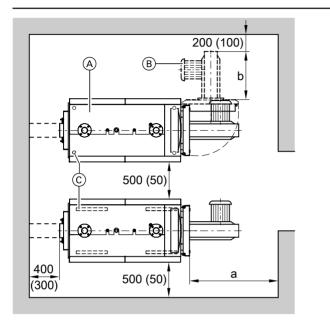
To enable convenient installation and maintenance, observe the stated clearance dimensions; maintain the minimum clearances where space is tight (dimensions in brackets). In the delivered condition, the boiler door opens to the left. You can reposition the hinge bolts so that the door can open to the right.
