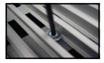
Using a 2.5mm Allen Key remove the M4 Flange Head Screws which retains the Top Grille.
