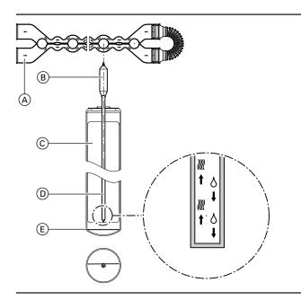
(A) Copper double pipe heat exchanger
